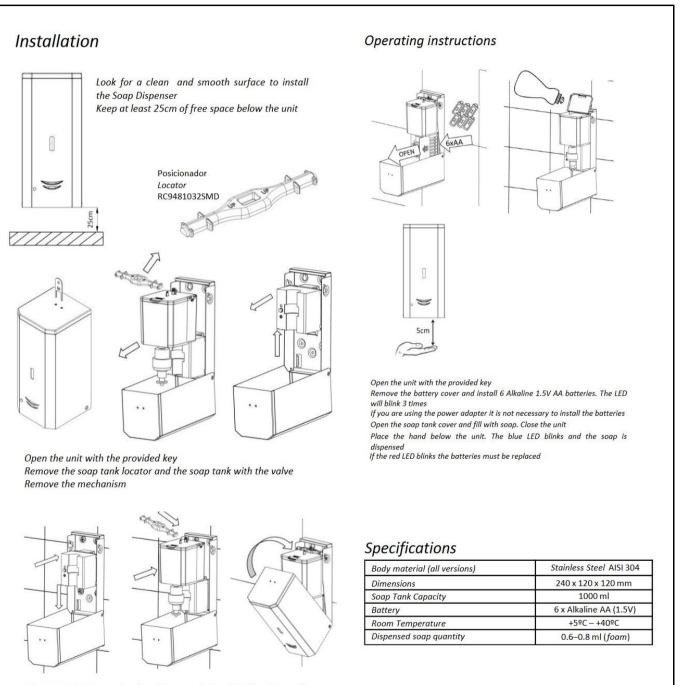
Reassembly the mechanism, the soap tank with the valve and the soap tank locator Close the unit
